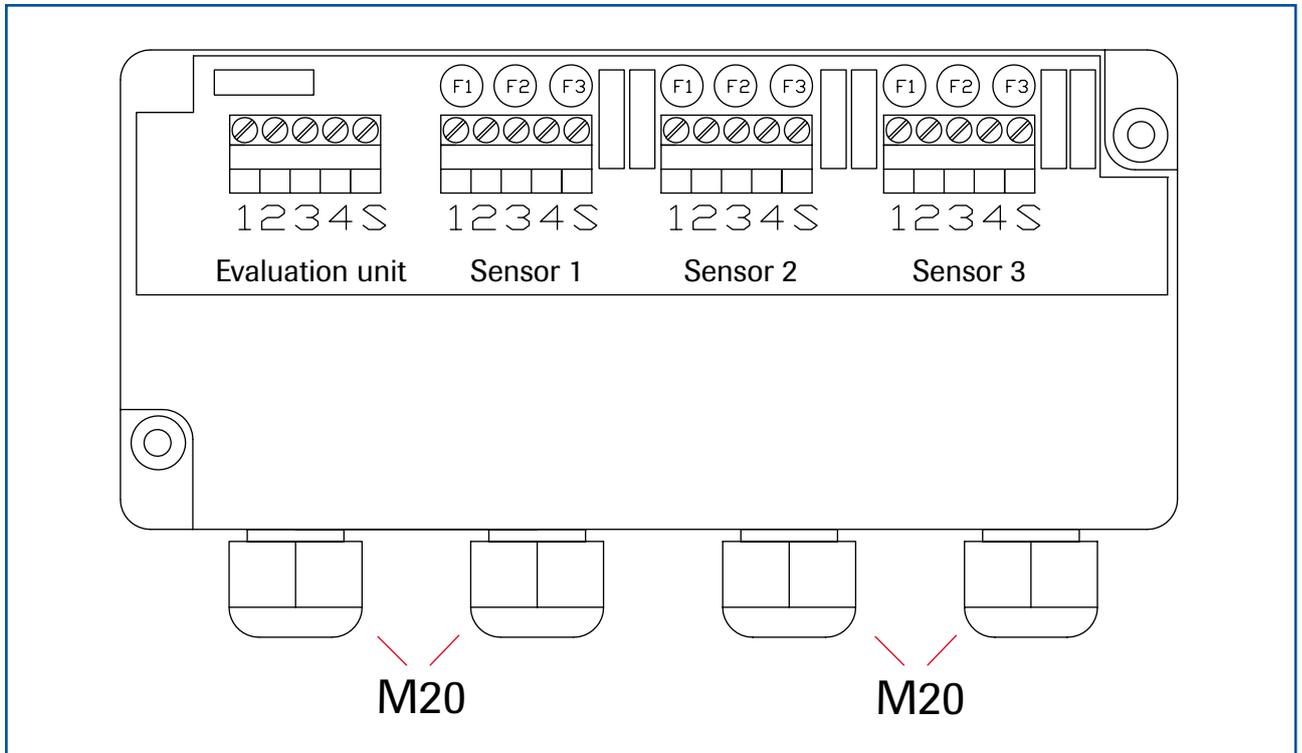
Fig. 16: Electrical connection for the C3-Box
