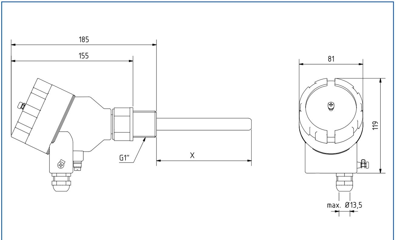
Fig. 12: Dimension of the PicoFlow sensor
