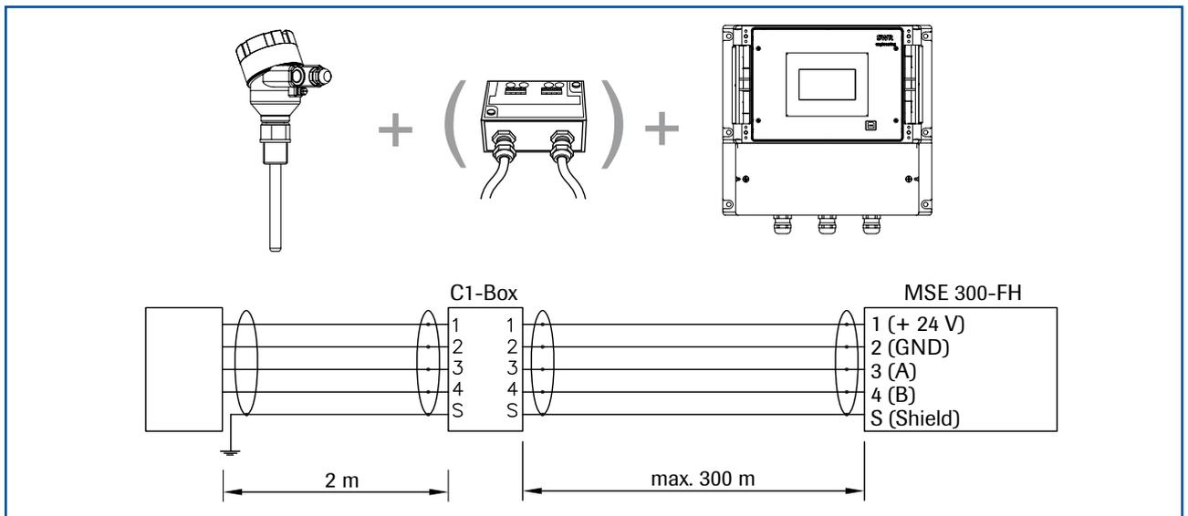
Fig. 1: Overview with C1-Box and MSE 300 in the field housing
