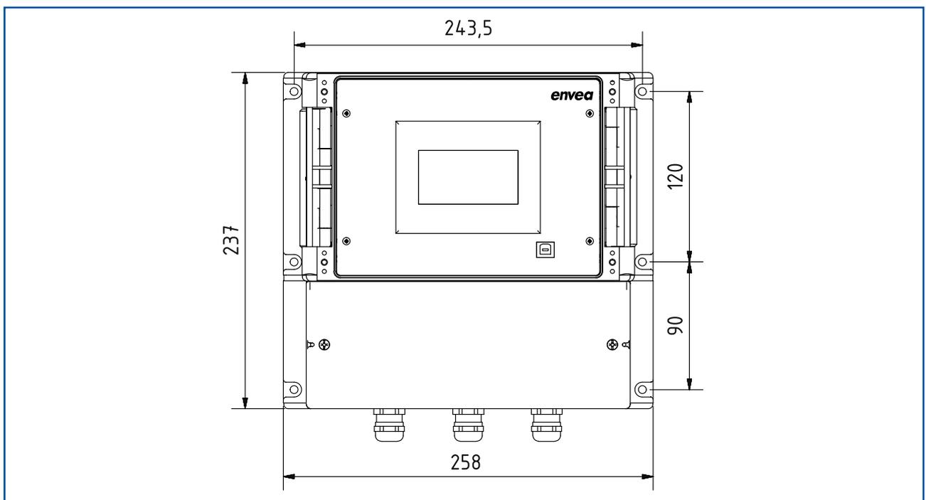
Fig. 8: Dimension of the MSE 300-FH (front)
