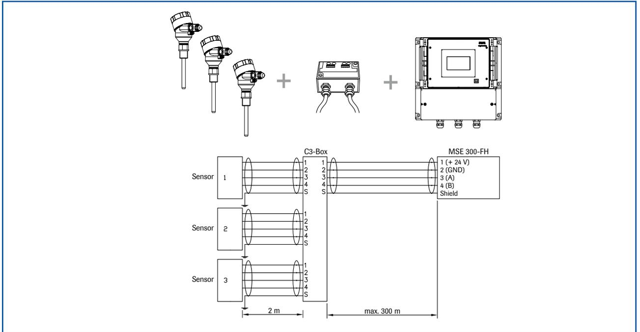
Fig. 3: Overview with C3-Box and MSE 300 in the field housing
